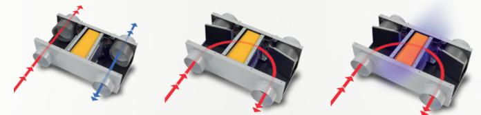
Blocking the outward airflow with the shutters and diverted to the special filter.
