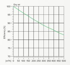
Efficiency as a function of the airflow
