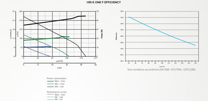
Efficiency as a function of the airflow
